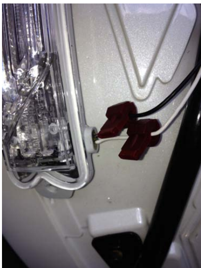
USING THE SUPPLIED T-TAP, SPLICE IN THE + AND - WIRE ON THE FRONT FENDER POSITION LED.
