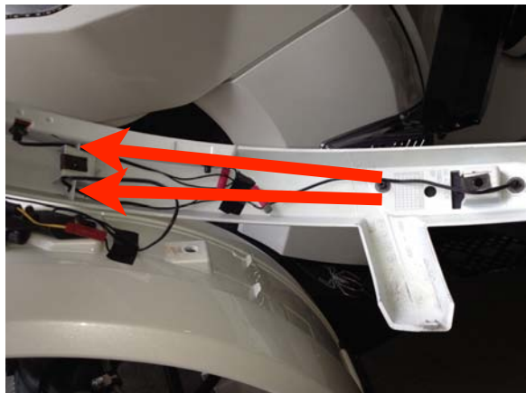
DRILL TWO HOLES JUST ON EACH SIDE OF THE CENTER OF THE FENDER WHERE THE MIDDLE SCREW IS LOCATED. YOU WILL ROUTE WIRES FROM BOTH LED REFLECTOR THROUGH HERE TO KEEP IT FROM BEING PINCHED WHEN THE FENDER IS PUT BACK. ANOTHER HELPFUL TIP, USE BLACK VINYL TAPE AND TAPE DOWN THE WIRES ON TOP OF THE FENDER TO KEEP THEM NEAT.
