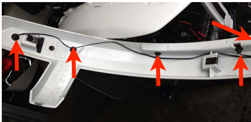
REMOVE THE 2 FACTORY REFLECTOR BY USING A SMALL FLAT HEAD SCREWDRIVER AND PRY OPEN THE PUSH-NUT HOLDING THEM TO THE FENDER. 5 TOTAL (EACH SIDE). WHEN DONE INSERT YOUR NEW LED MARKER LIGHT. NOTE LH AND RH SIDES MARKED ON THE BACK OF EACH LED REFLECTOR. SECURE BOTH LED REFLECTOR USING THE NEW PUSH-NUT PROVIDED.
